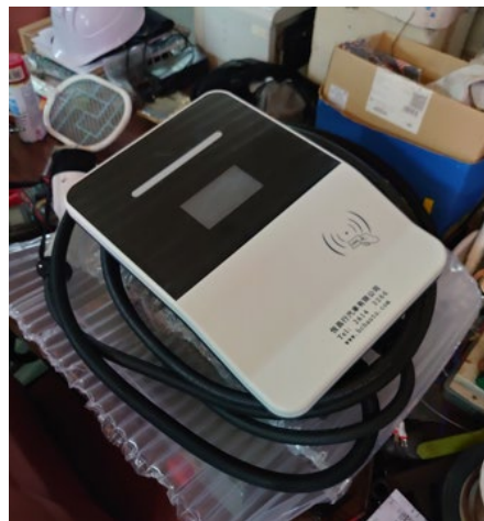
22 kW three-phase AC charger (Carried by the EV)
