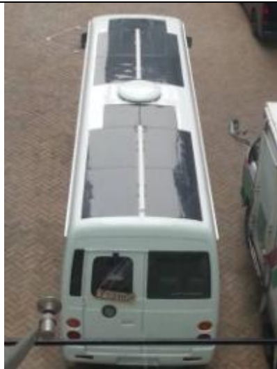
Solar panel, part of the SAS, on SAV roof
