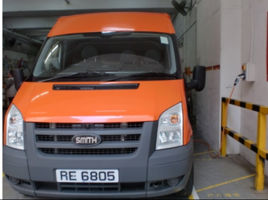
EV charging from the charging socket
