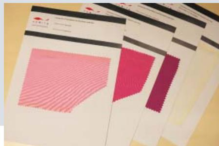
Textiles made from conversion of food waste into polylactic acid fibre
